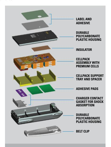
Every component of our battery is built tough from the inside out. We start with premium cells, add shock absorbing spacers and materials and complete the design with a durable polycarbonate plastic housing. Even the belt clip is designed to absorb some impact when a battery is dropped. Finally, we complete our battery design with state-of-the-art computer-controlled assembly equipment. All of this is done to help ensure you have a battery that performs in even the toughest conditions.
